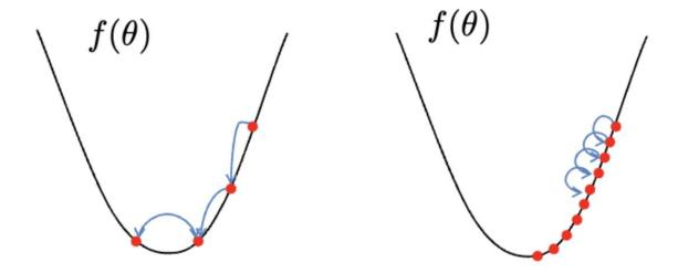
Large  $a \Rightarrow$  Fast convergence but larger residual error. Also possible oscillation. Small  $a \Rightarrow$  Slow convergence but small residual error.
